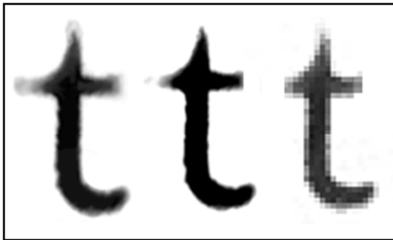
Figure 15. Letter “t” scanned in and artificially “worn” out; printed in high contrast; then rescanned in 72 pixel/inch resolution. Results are identical to comparable characters in the Bush memo.
