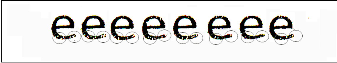
Figure 13. Damage can often become more apparent at high contrast. While the bottom of the characters show consistent damage, the left side of the bowl on the fourth “e” from the left shows damage caused by a defect in the ribbon or paper.
