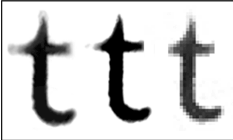
Figure 11. Letter “t” scanned in and artificially “worn” out; printed in high contrast; then rescanned in 72 pixel/inch resolution. Results are identical to comparable characters in the Bush memo.
